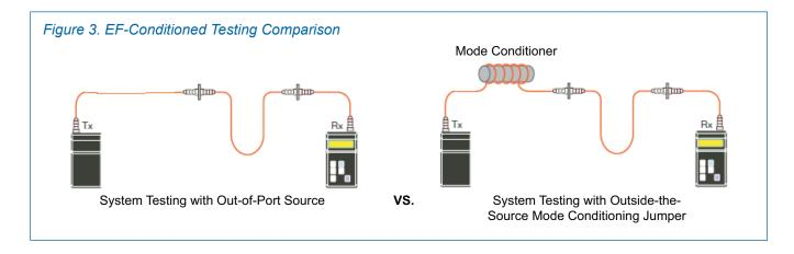
Corning Cable Systems believes that EF is the most accurate method to test multimode fiber. An EF-conditioned launch will reduce the variability among sources today (+20/-40 percent) to the respectable +/- 10 percent variability, and it will provide the best system characterization for 1 Gb/s and beyond.
